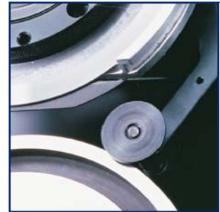
Adjustment slide Simple adjustment to bottom knife
